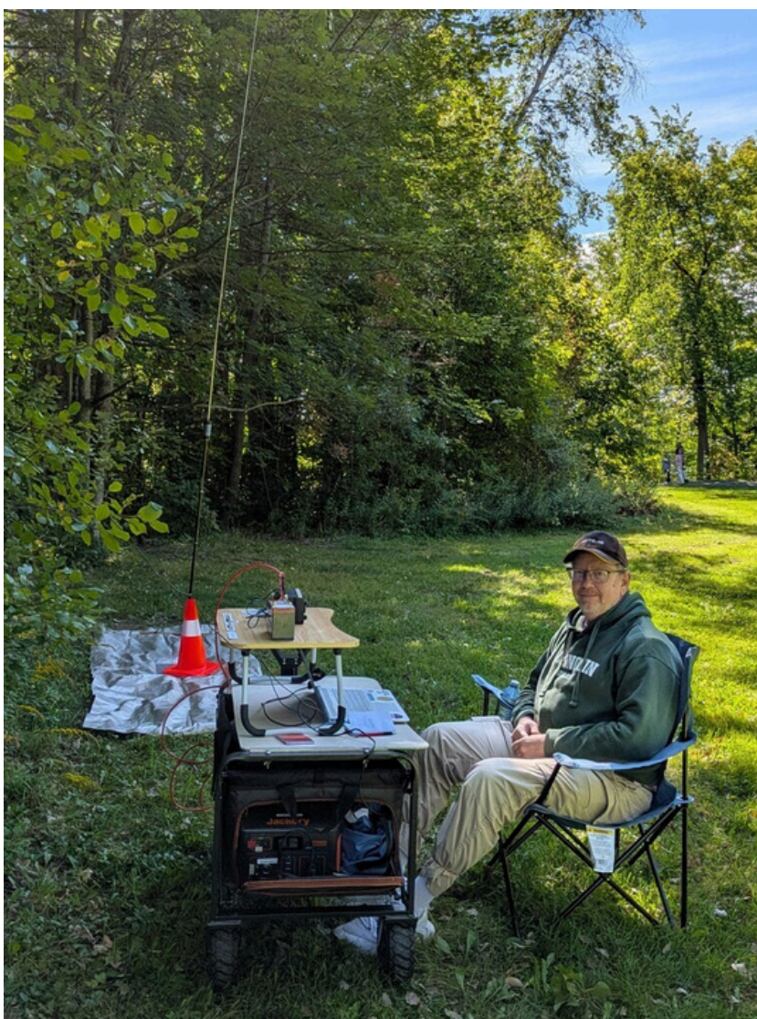
Photo 1: Steve (VE3MVK) set up and operating on 20m with his Icom 705 and vertical antenna.
