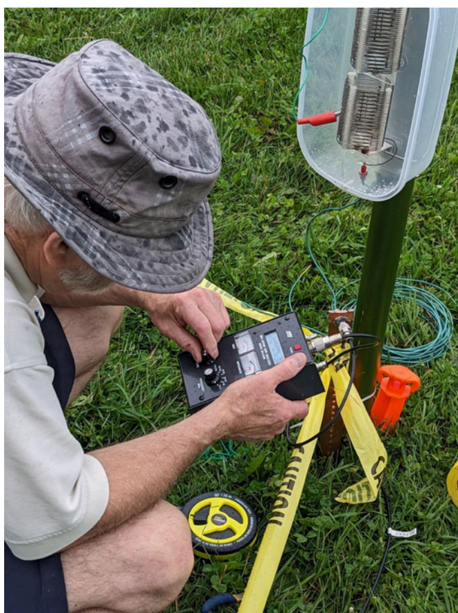
PHOTO 3 - NORM, VE3LC, ADJUSTING THE LOADING COIL TO TUNE UP THE 43 FOOT VERTICAL FOR 80M.
