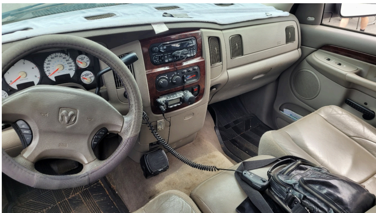
Photo 10 - Yaesu 857D remote control head mounted in the centre console of Pete, VE3XEM's truck.
