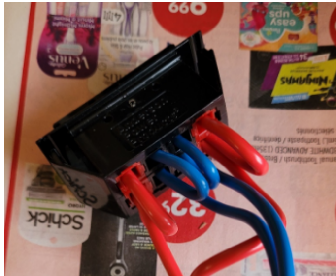
Photos 20 - 25 - Sub-harness complete for the PowerPole outlet.
