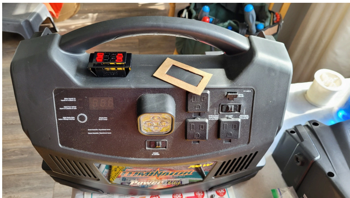
Photo 9 - my used MotoMaster Eliminator power box showing the Powerwerx four outlet PowerPole receptacle before mounting.
