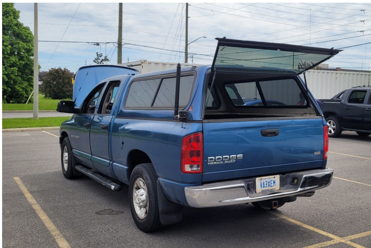
Photo 8 - Pete, VA3XEM/VE3XEM, has a Yaesu ATAS 120A HF/VHF screwdriver style antenna mounted on the back of his truck and a separate VHF antenna on the hood.
