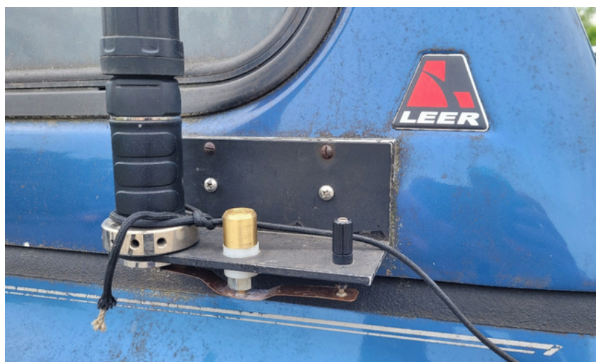
Photo 8 - Pete, VA3XEM/VE3XEM, has a Yaesu ATAS 120A HF/VHF screwdriver style antenna mounted on the back of his truck and a separate VHF antenna on the hood.
