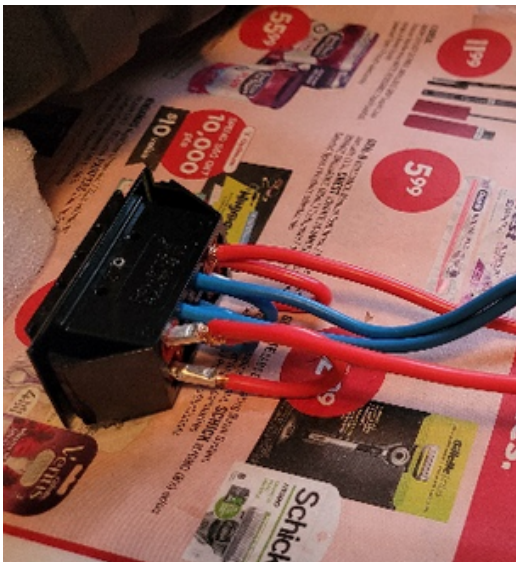
Photos 20 - 25 - Sub-harness complete for the PowerPole outlet.
