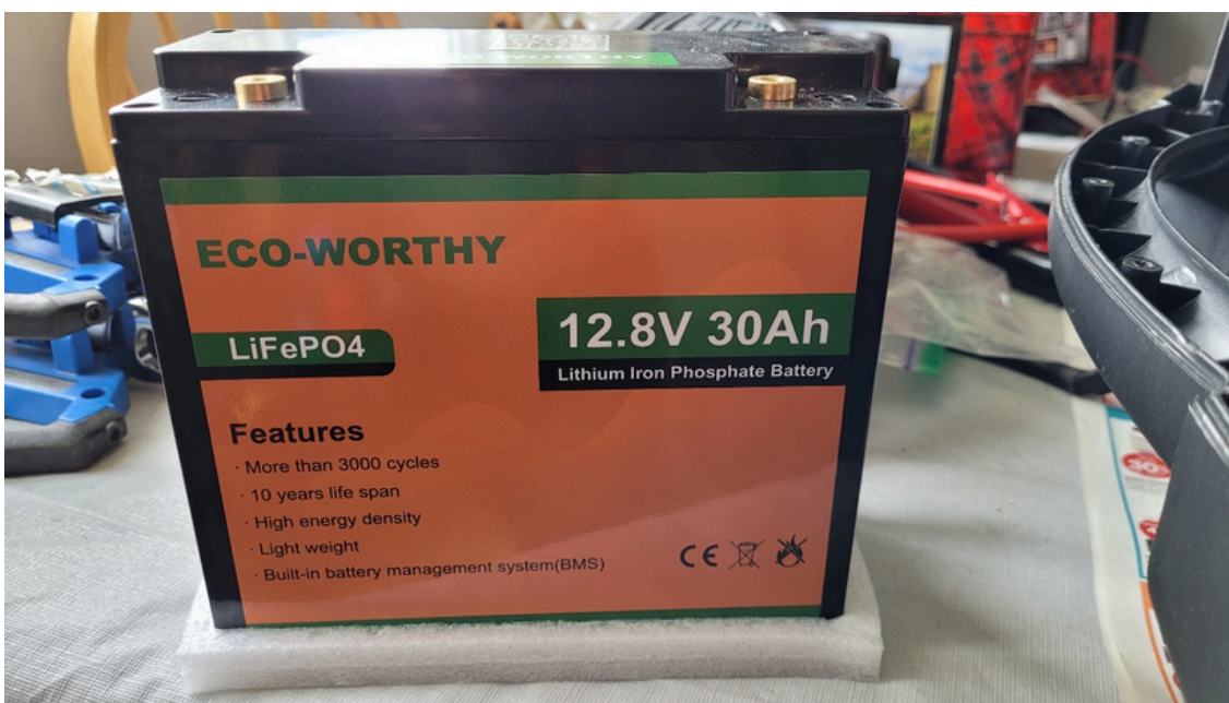
Photo 17 - Eco-worthy 30 Ah LiFePO battery.
