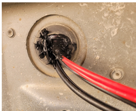
Photos 10 and 11: The access point grommet was partly cut out to allow the cables to access the cab and then well sealed with Black Silicone sealant.
