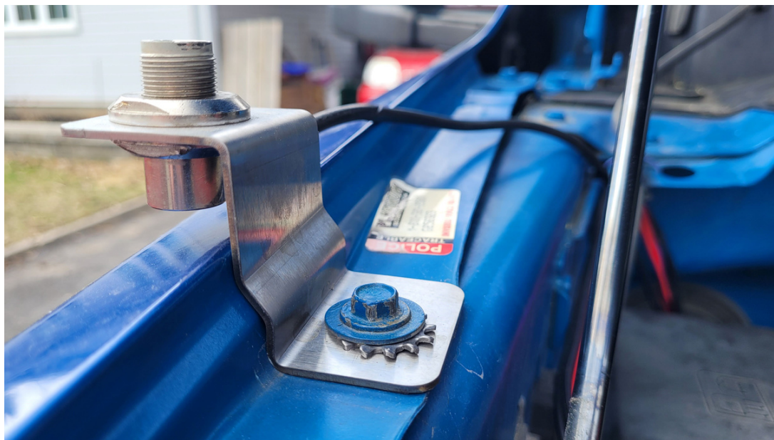
Photo 1: Comet fender mount in place, showing how it follows the contour of the fender and uses the existing fender bolt to hold it in place. The star washer on top of the antenna mounting bracket bolt improves the ground connection. Also in the pic is the SO239 type right angle connector with the coax running back towards the firewall.
