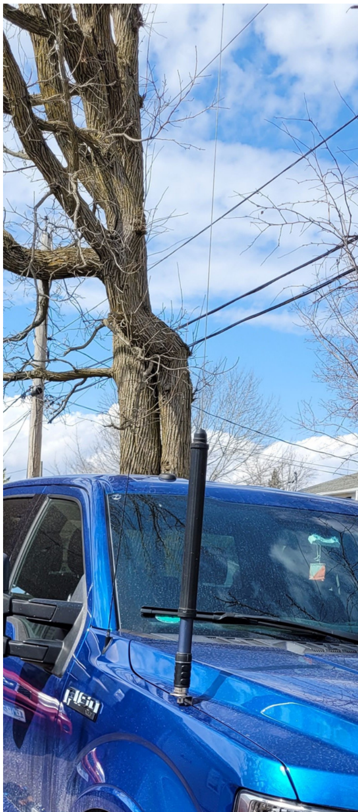
Photo 7: ATAS installation and power cables completed.
