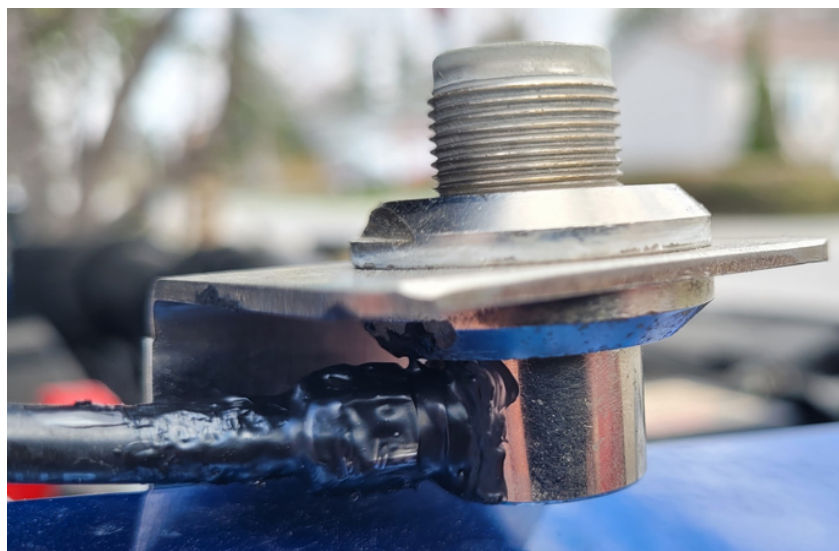
Photo 1: Comet fender mount in place, showing how it follows the contour of the fender and uses the existing fender bolt to hold it in place. The star washer on top of the antenna mounting bracket bolt improves the ground connection. Also in the pic is the SO239 type right angle connector with the coax running back towards the firewall.
