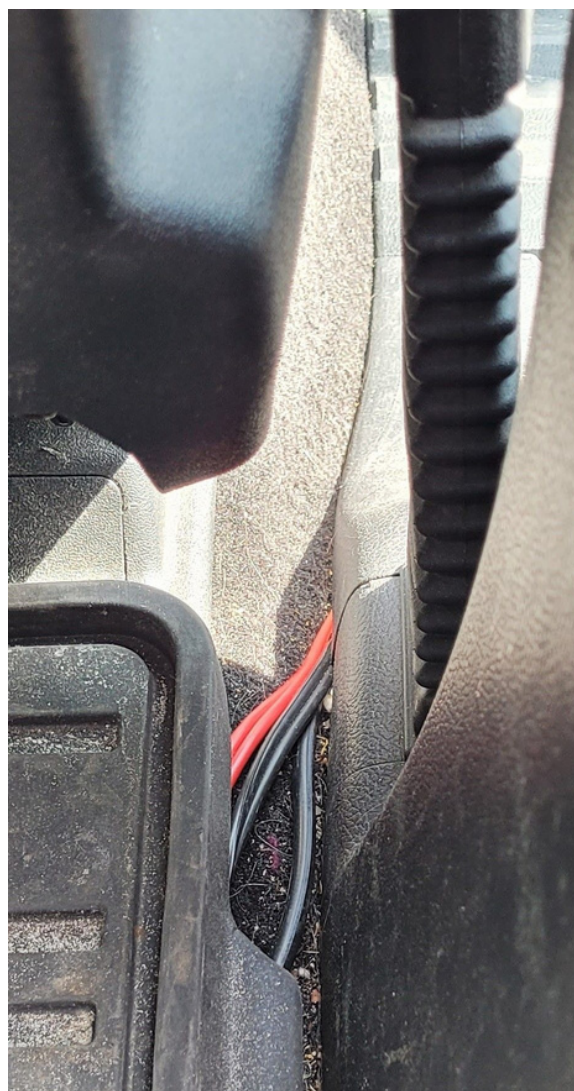
Photos 10 and 11: The access point grommet was partly cut out to allow the cables to access the cab and then well sealed with Black Silicone sealant.
