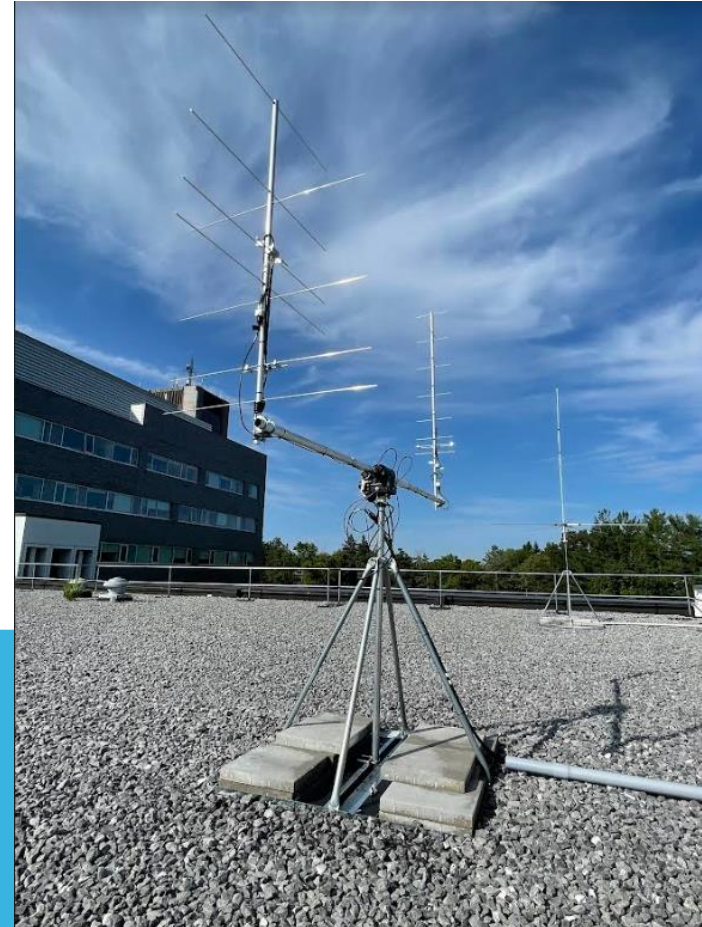
M2 LEO-Pack Dual Yagi Antenna System 2M/70cm with AlfaSPID Rotator for Satellite Communications
