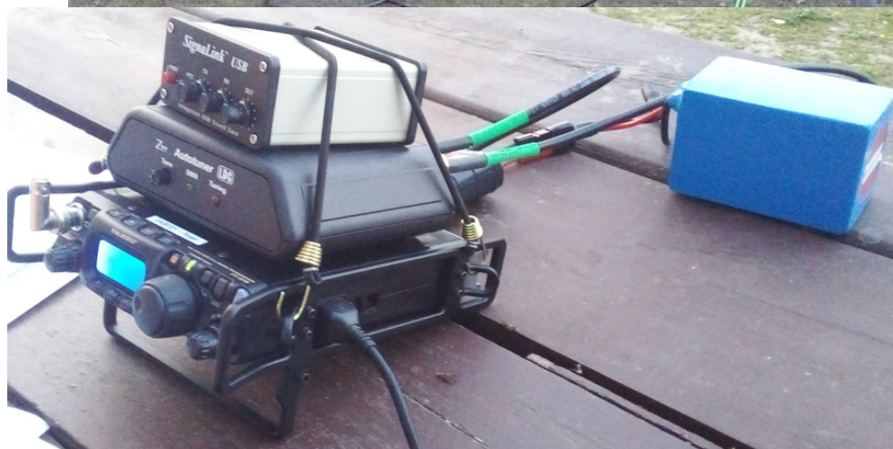
VA3EGY, Roger's portable setup of a Yaesu FT-818 with LDG 817 tuner and Signalink powered by a Bioenno LiFePO battery.
