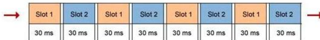
Tier II TDMA 30ms Time Slots
