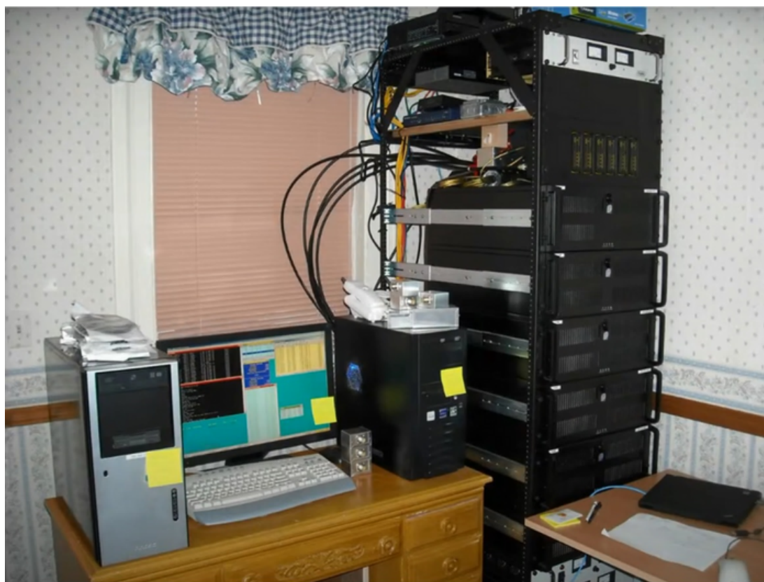
Figure 3: First generation K3LR CW skimmer hardware with six rack mounted servers, six Perseus SDR HF receivers and custom server power supply. Image credit K3LR)
