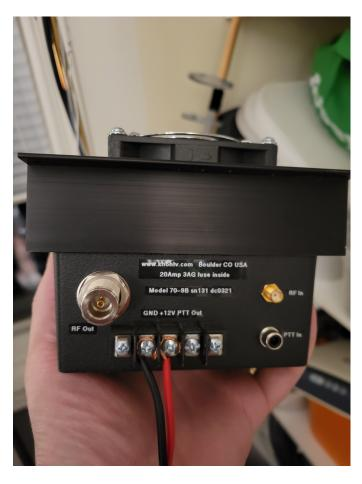
The Power Amplifier (PA) is from Jim KH6HTV model 70-9B. This is a 70 watt wide bandwidth amplifier that is useful for DATV signals.
