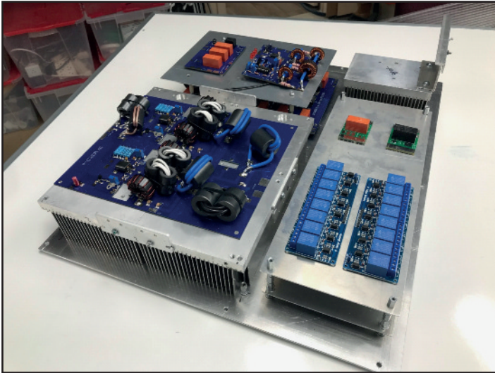
Side view of the inner structure of the amplifier module.
