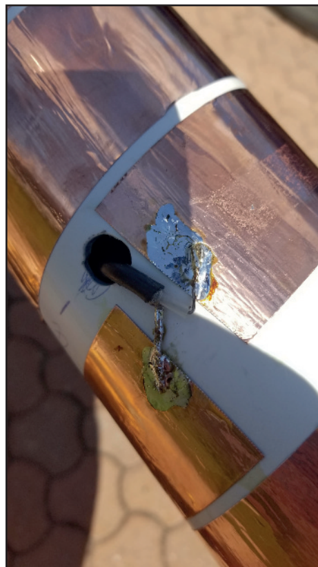
Figure 2 - Soldered centre coax feed point.
