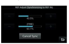
Menu screen showing the automatic adjustments to compensate for frequency drift of TCXO based on the 10 MHz reference signal input.
