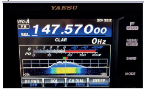
display which shows a clean signal and a strong ERP with antenna gain.
