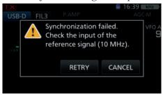
If the GPSDO 10 MHz signal is lost to the IC- 9700, it flashes up this message.
