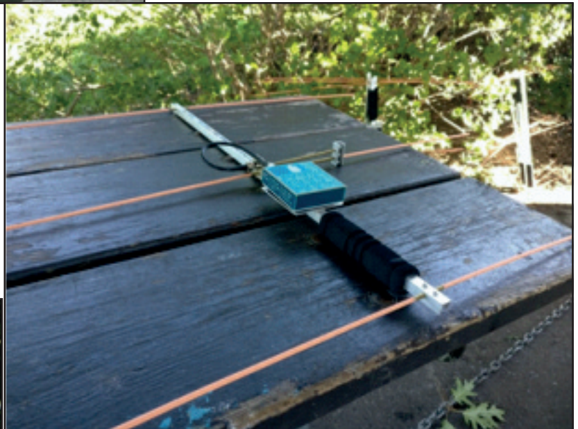
A 3 element Yagi and Sniffer 4 all set to go find the 'fox'.
