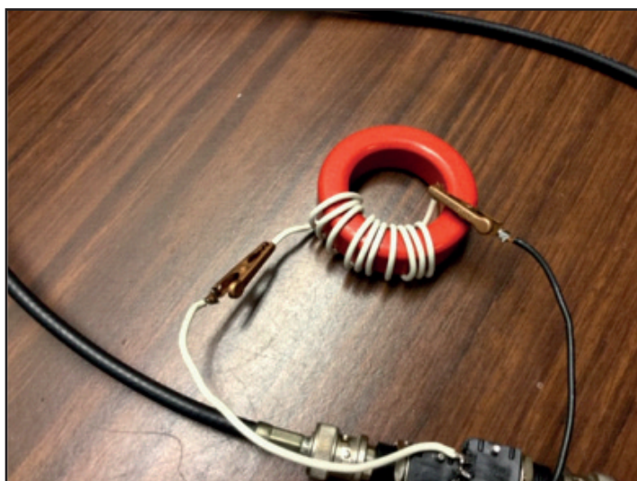
Surplus Toroid Core colour coded RED – Under Test – 10 turns
