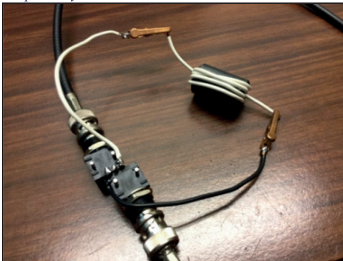
Similar response from previous toroid core. Attenuation increases with frequency.
