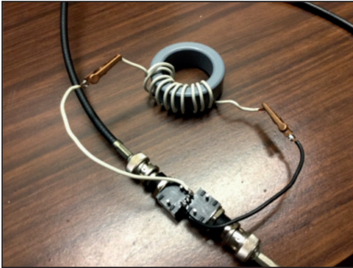
Surplus Toroid Core colour coded GRAY – Under Test with 10 Turns
