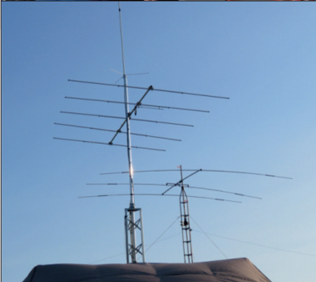
5 element 6 mtr beam for FT-8
