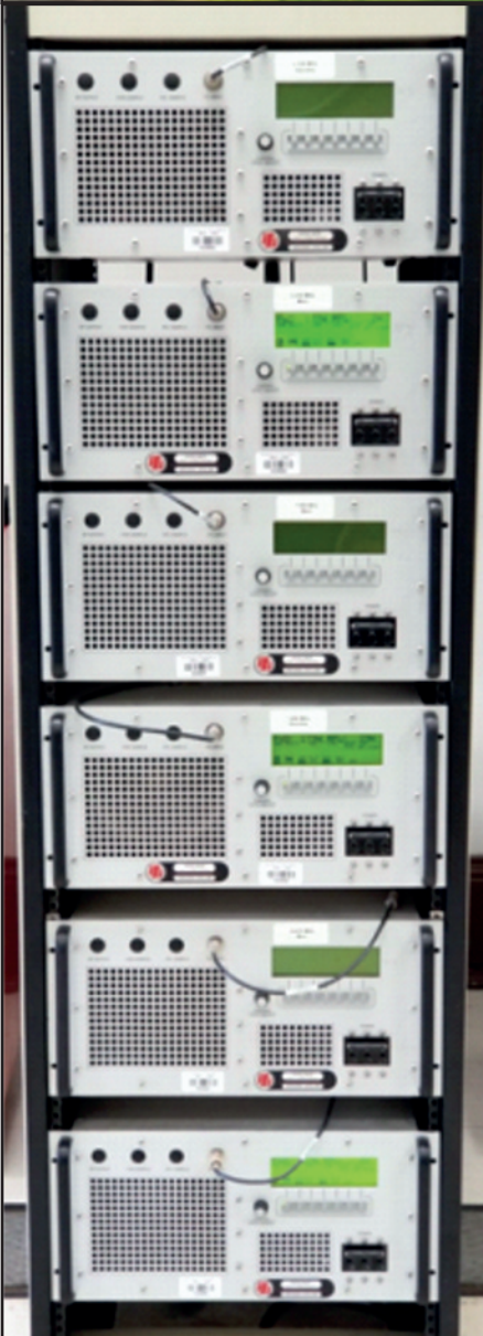
Bank of main and standby solid state exciter amplifiers made by IFI (Instruments for Industry, Ronkonkoma, NY).
