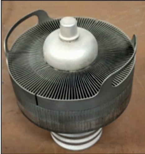
4CX 10000 Ceramic RF Tetrode on display from one of the CHU transmitters.
