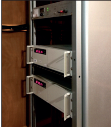
High accuracy Cesium Beam Atomic Clocks keep CHU on time and on Frequency. Clocks are installed in an RF tight "Screen Room" to insure the RF from the Transmitters doesn't upset the clocks' operation.
