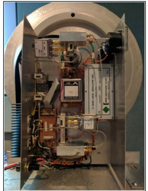
Inside Ray's home brew microwave station equipment showing individual components.
