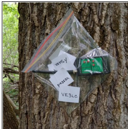
One of the hidden transmitters - 1 mW on 145.000 Mhz
