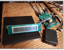
measuring RF power and SWR of QRP SDR transceiver. Display is indicating 20 metre band, Forward Power 1.023 watts and SWR 1.0 to 1 (it's into a 50 ohm load).
