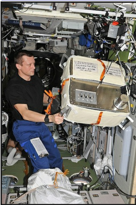
ARISSat-1 on board the ISS in storage garb. The control box is on the left side and the Kursk University (Russia) experiment (protruding) to measure vacuum in space, on the lower right side.
