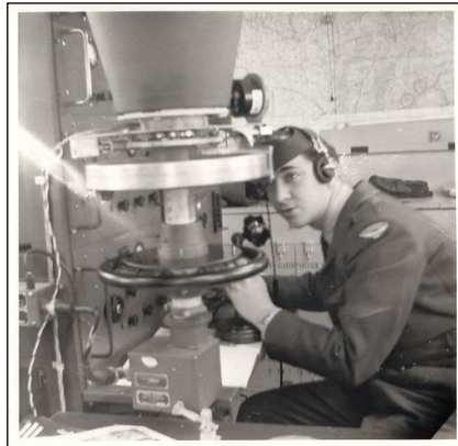
Figure 2: The inside view shows the manual rotor wheel used to spin the antenna consisting of two driven elements and two reflectors. In the middle of the wheel is a round black plate which we depressed in order to establish if we had a direct bearing or a reciprocal. We would read off the bearing indicated on the 360 degrees scale above the manual rotor wheel. The radio used was a BC-639 VHF unit tuned to air navigation frequencies.
