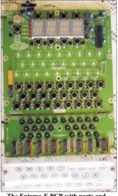
The Enigma-E PCB with parts and plexiglass lamp board.
