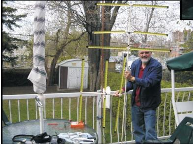
You can see the result in this picture. I was invited at Gerry's home with the Club's MFJ-259 Analyzer to help him put the final touches on the tuning of the antennas. After straightening a few elements and connecting the 259 we found the antennas to be resonant at very close to the middle of 2m Amateur Radio band. Minor adjustment to the tuning stubs and all was perfect.
