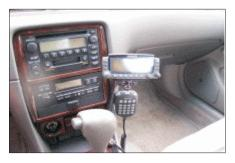
The mount is a very solid. heavy gauge metal bracket that makes use of existing screws in my dash. In the case of the Camry I pop off the center trim, undo two screws used to attach the climate control, put in the PanaVise bracket and screw the thing down
