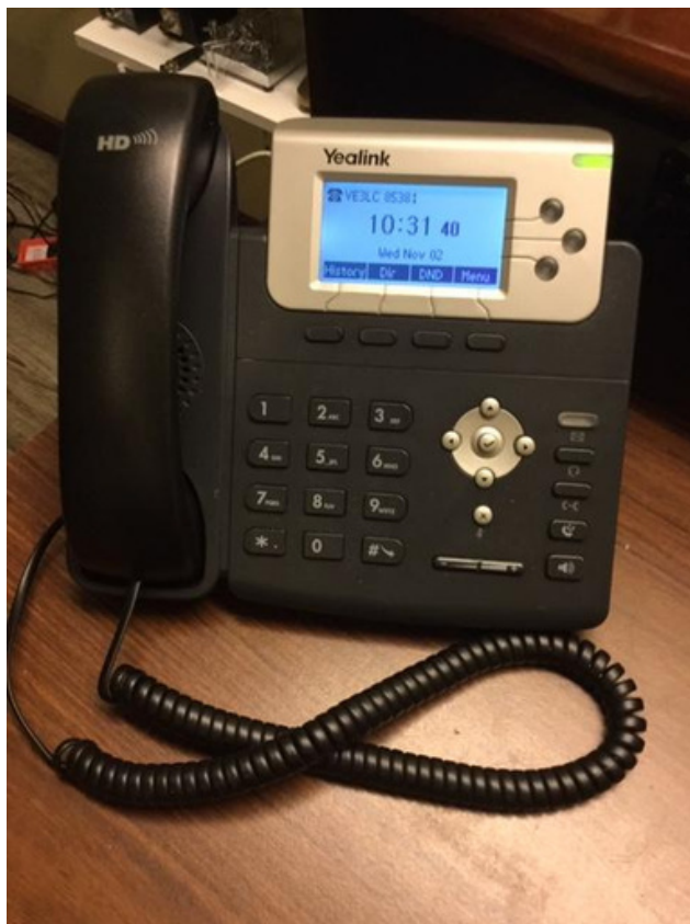
Here's another HH phone I have in the shack; it is a Yealink T22P. Although this phone is not on the HH supported list, it was easy to configure for use on the HHUX experimental server and works well on the system. This phone is factory reset by holding down the centre button with the check mark for 10 seconds.
