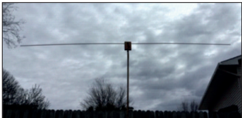
The 6 metre dipole mounted atop a \frac{3}{4} inch diameter wooden pole ready to intercept some 50 MHz signals.
