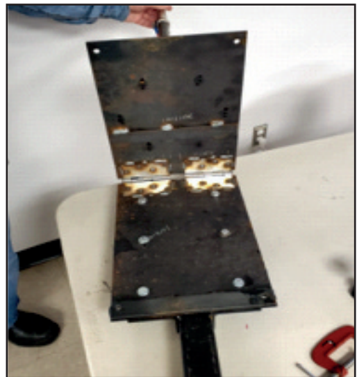
Denis, VE3BF's custom made fold over trailer hitch mount for his Valcom 35 foot vertical portable antenna.
