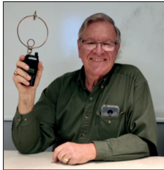
Peter, VE3XEM shows off this home brew 2 mtr mag loop antenna for DF'ing
